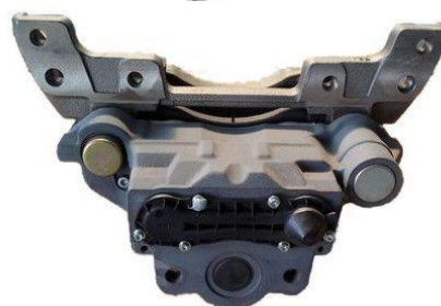
Knorr brems 6 Series Right hand CSL6558 19.5" Wheel
